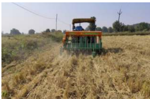
Fig. 1: Sowing of wheat with happy seeder and zero tilled wheat crop (WB 2)
