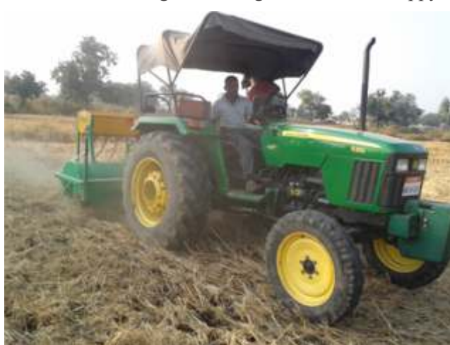
Fig. 2: Sowing of summer greengram with happy seeder and zero tilled crop (IPM 02-03)
